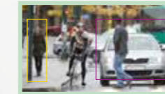
Human/vehicle classification Helps reduce false alarms by detecting and recognising people and vehicles.
