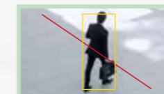
Line crossing detection Triggers an alarm if a person or vehicle crosses a virtual line.
